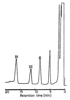
FIG. 1. Gas chromatogram of authentic salicylates as their trimethylsilyl derivatives. I-m-toluic acid (internal standard), II-SA, III-ASA, IV-salicylamide.
